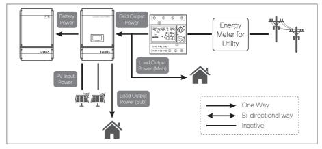
[Figure 3-7: Grid Charge Mode]
