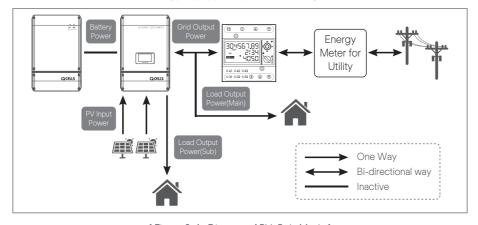
[Figure 3-4: Diagram of PV-Only Mode]
