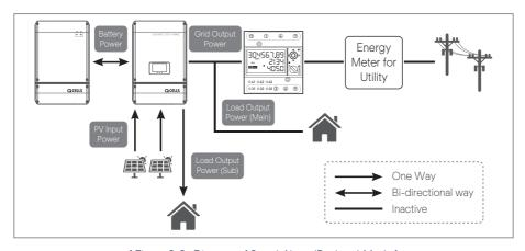
[Figure 3-6: Diagram of Stand-Alone (Back-up) Mode]
