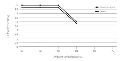
[Figure 2-1: Derating Curve]
