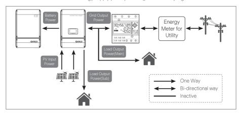
[Figure 3-2: Diagram of PV-Auto Strong Mode]
