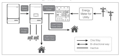
[Figure 3-5: Diagram of Battery-Discharge Mode]
