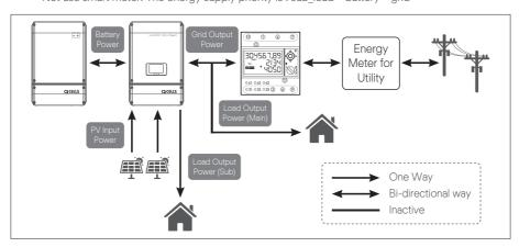
[Figure 3-3: Diagram of PV-Auto Strong Both Mode]
